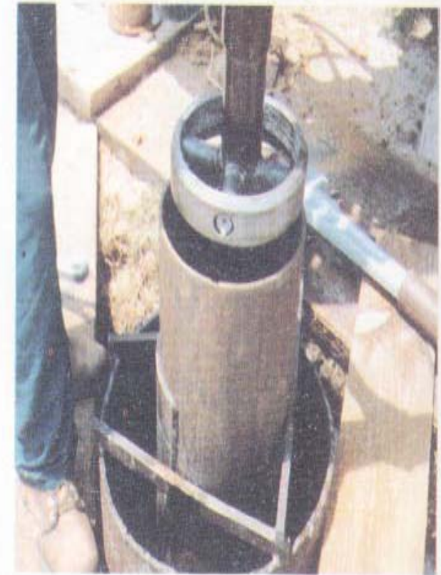
Figure 15.17. Four-nozzle jetting tool designed for jet development of well screens. The check valve allows the jetting tool to be used for intermittent pumping of the well. A plate bottom is often used in place of the check valve if the tool is not to be used for pumping. To avoid breakage, the pipe base of the tool can be made of heavy-wall pipe if it is to be attached to the bottom of the drill pipe. At right, a jetting tool is being lowered into inner casing that has been centered in the surface casing.
